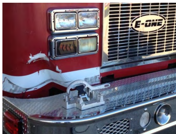
Figure 2 Reserve Vehicle 1249 Front Chassis Damage (behind bumper)
