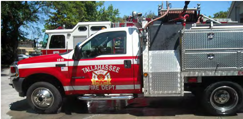
Brush (Vehicle 1315) - These are usually trucks with off-road capabilities for traversing rough terrain in order to reach the fire.
