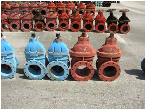
Example – System Gate Valves (10 inch)
