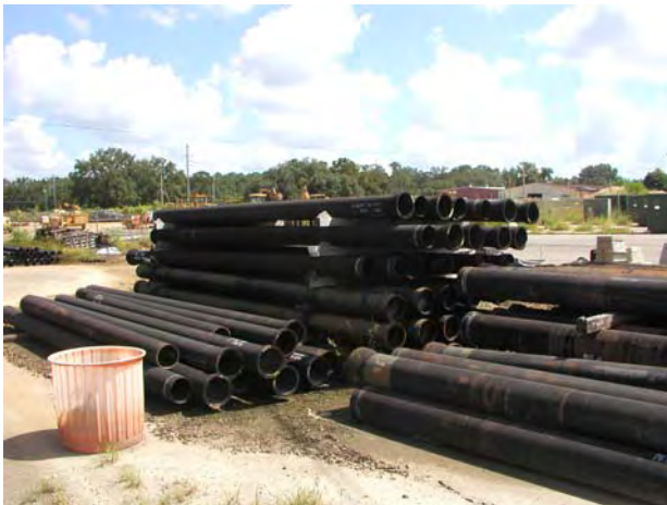
Example – Ductile Iron Main - 20 foot sections (8 inch)
